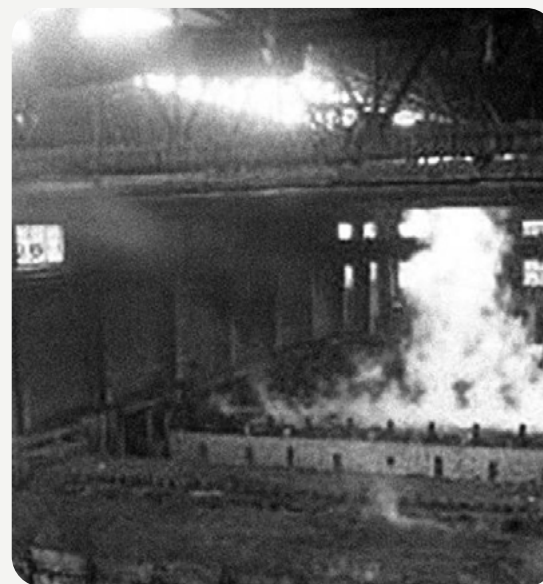
↑ Synthetic graphite is today produced using open Acheson furnaces, with a high CO 2 footprint
